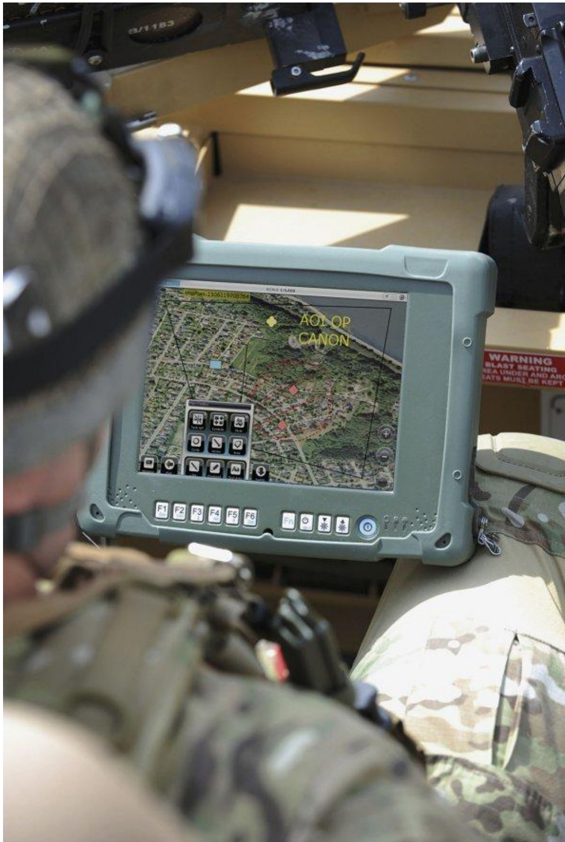
Systematic Frontline hosted on a Roda Panther DR8-M tablet, showing a graphic overlay on satellite imagery and the soft function keys. (Copyright © Systematic) 1357000
