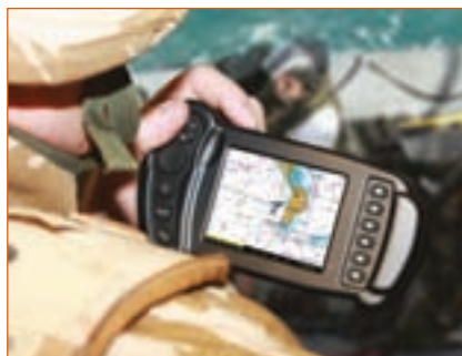
Cobham's Marinised Data Terminal, showing WaveHawk C2 software being used with an electronic chart. (Photo: Cobham)
