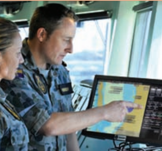
The Saab 9LV Situation Awareness Terminal mounted on the bridge of a frigate. (Photo: Saab)
