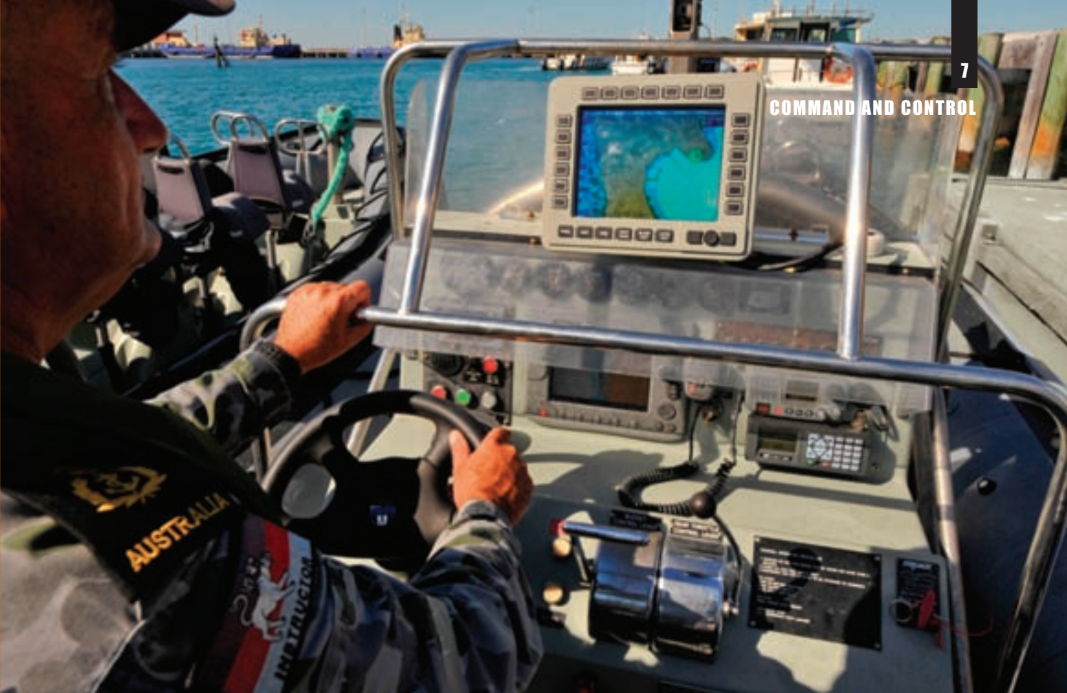
The Royal Australian Navy has equipped its RHIBs with Saab 9LV SAT terminals. (Photo: Saab)
